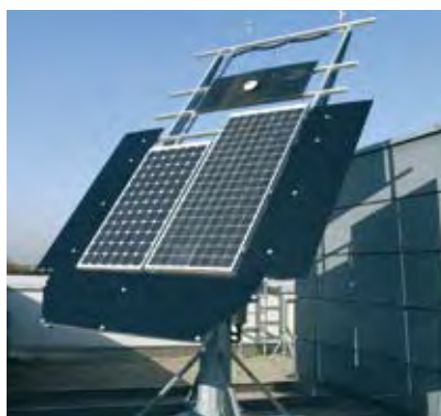
Fig. 1: Outdoor test stand to determine the "nominal operating cell temperature" (NOCT). The single-axis tracker allows the required testing times to be shortened.
