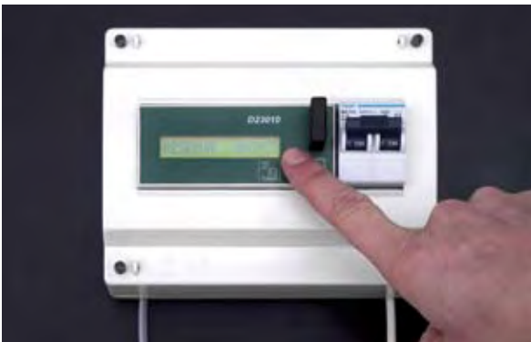
Fig. 2: The Energy Dispenser distributes a certain amount of energy per day. If a large amount of energy is available to the system (e.g. during sunny periods), the users can consume twice as much energy for the same price. Conversely (e.g. during the night, when the battery capacity is almost exhausted), only half as much energy is supplied for the same price. We replaced its proprietary communication bus by a universal CANopen interface with standardised commands for input and output devices.
