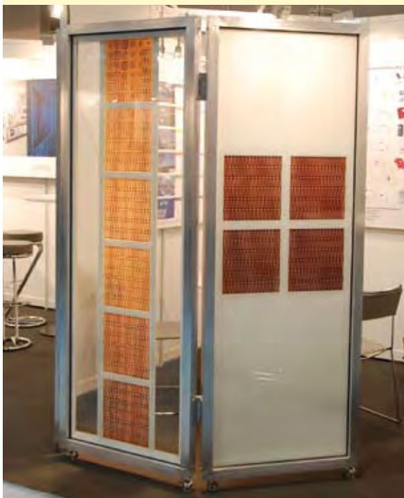
Fig. 1: Demonstration unit for trade fairs – constructed of several dye solar cell modules (30 cm x 30 cm), which are laminated between panes of architectural glass. Different options for integration into the building envelope are shown: lamination of semi-transparent modules in a glazed façade (left) and integration into a ventilated façade (right).
