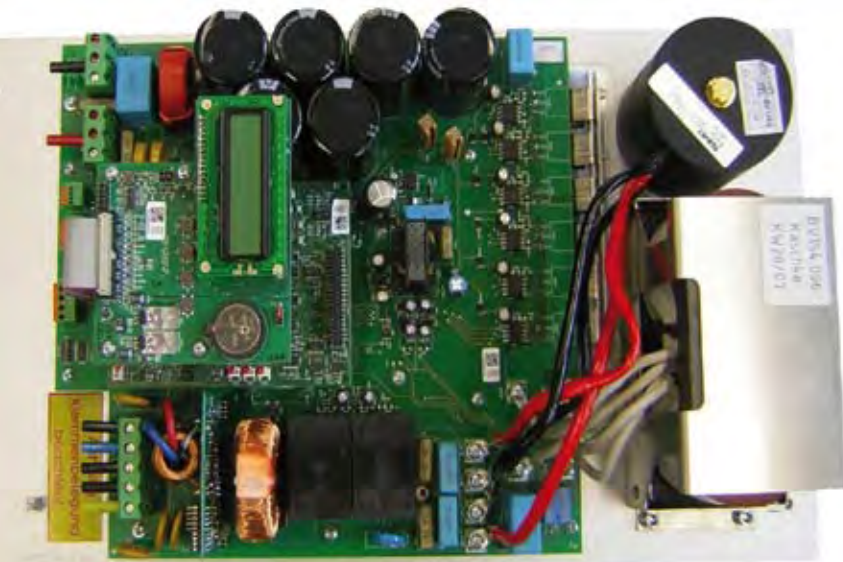
Fig. 1: Single-phase PV inverter with HERIC® topology, 5 kW rated power, 350 V intermediate circuit voltage and 16 kHz switching frequency. The development was commissioned by an industrial partner.
