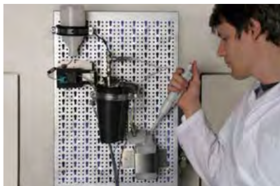
Fig. 2: Experimental set-up to test different reactor types in a hydrogen generator based on chemical hydrides. It consists of a storage vessel, a dosing pump, a thermally insulated reactor and a collection vessel. Exact knowledge of the possible reaction paths during the release of hydrogen is needed for optimal dimensioning of the system.
