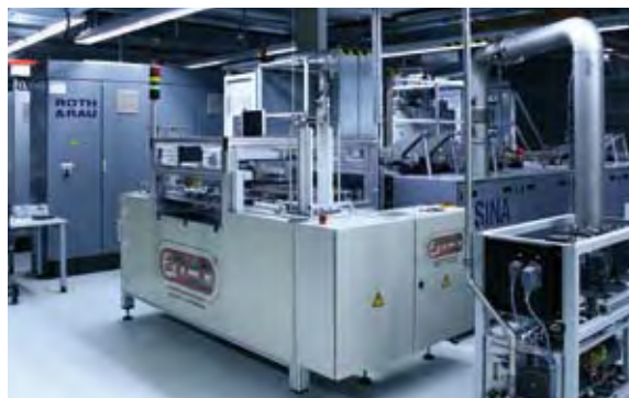
Fig. 2: Automated, industrial PECVD unit for in-line deposition of amorphous silicon, silicon nitride and silicon dioxide.
