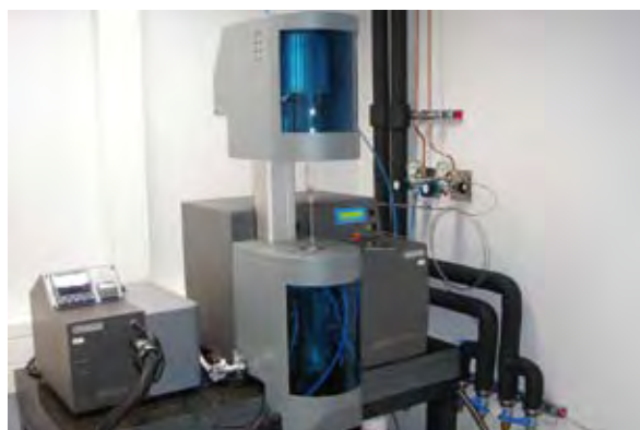
Fig. 1: Autoclave with stirring accessory for synthesis of highly porous sorption materials in the new synthesis laboratory.
