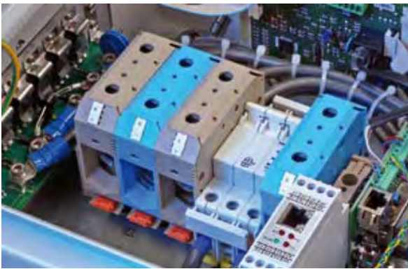
Fig. 1: "Tarom" PV charge controller from the Steca company for 24 V / 70 A with a UESP interface. The UESP interface consists of a small embedded system from the SSV company with a 32-bit coldfire processor (to the lower right of the photo). Fraunhofer ISE has implemented the UESP protocol including the network management under the Linux operating system in this interface. The same embedded system is used for the CANopen interface of the Energy Dispenser (Fig. 2).
