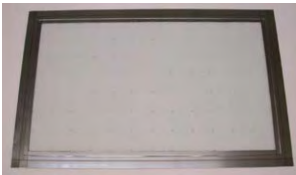
Fig. 1: Display sample of evacuated insulating glazing with a glass/metal edge seal (before edge polishing and framing) and glass spacers.
