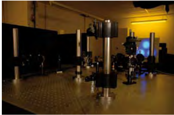
Fig. 3: Optical set-up for three-beam interference lithography. A laser beam is split into three equally intense beams, which are expanded and then superimposed on a photoresist-coated sample. The resulting interference pattern has hexagonal symmetry.
