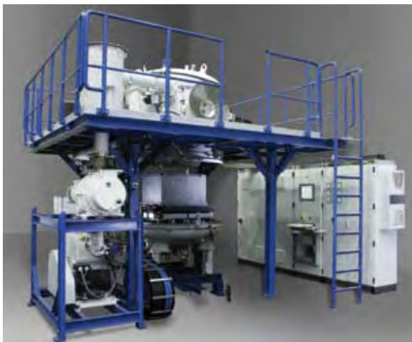
Fig. 1: Our system (height = 3.5 m) for the crystallisation of multicrystalline silicon ingots, which is close to the current standard in the photovoltaic industry. It features great flexibility: We can produce ingots in variable sizes with a base area of app. 20 x 20 cm 2 up to 68 x 68 cm 2 . Several sets of heating elements allow us also to crystallise and characterise silicon of very different quality grades.
