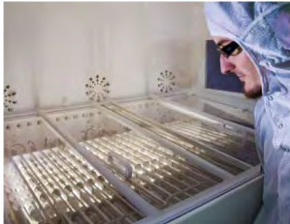
Fig. 1: In-line galvanisation unit at Fraunhofer ISE. The light sources in the bath are clearly visible.
