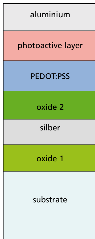
Fig. 1: Schematic stack structure of an organic solar cell with a transparent silver electrode
