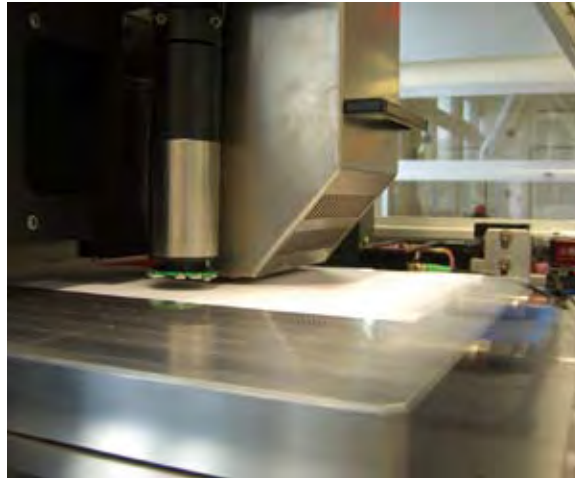
Fig. 1: Precise ink-jet unit at Fraunhofer ISE for printing silicon wafers with hot-melt pastes. The system is able to operate with different pastes and printing head modules. In addition, a simpler printing system is available, with which new pastes and printing heads can be tested, before they are transferred to the main unit.
