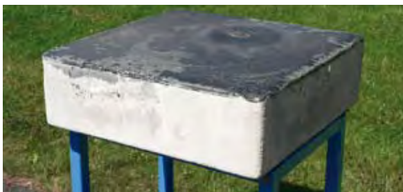
Fig. 2: Crystallised silicon ingot of highly doped "tops and tails", waste material from the microelectronics industry. The ingot has a base area of app. 68 x 68 cm 2 , and with a height of app. 25 cm, weighs about 270 kg.
