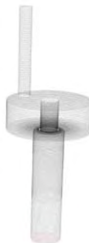
Fig. 1: The discretised reactor geometry, with its mixing chamber, reaction zone (catalyst) and outlet zone, serves as an input file for the actual CFD simulation. The image shows the grid over an auto-thermal kerosene reformer, in which a mixture of air and water vapour is introduced via the upper pipe. This mixture is fed into the reactor chamber via an annular gap. We feed liquid kerosene centrally in the annular gap via a single-component injector.
