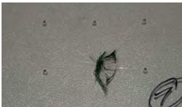
Fig. 2: Damage to an experimental sample caused by impact from a steel ball. The glass breaks at the position of these spacers, which were thus classified as unsuitable.
