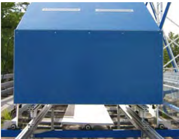
Fig. 3: Equipment to measure the form compliance of narrow reflectors. Here it is being used to measure a reflector for the demonstration collector of PSE GmbH in Freiburg. The compliance of the reflecting component form with specifications is tested.
